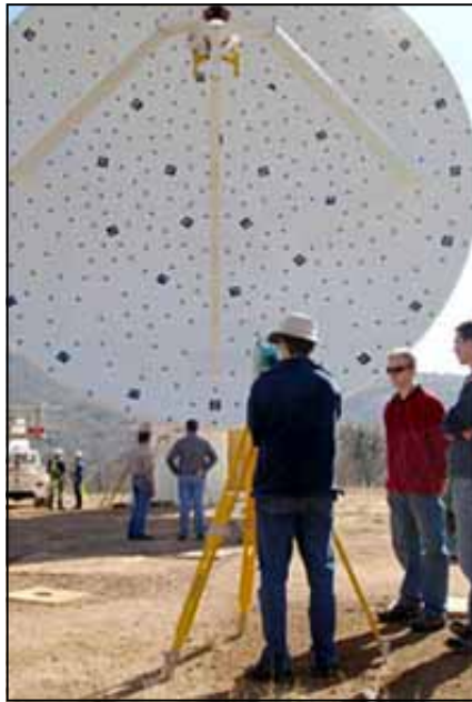
Fig 1: Theodolite and Photogrammetry measurements.
