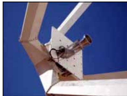
Fig 2: The 1.42 GHz (left) receiver fitted on the dish. On the right Pieter Stronkhorst is busy fitting the 12 GHz receiver.
