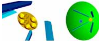
Figure 1: The five conical covers, two horns, feed cluster backplane (all in yellow), and top sections of the four struts (light blue) are shown on the left. A zoomed-out view is shown on the right, with the floodlight illuminator and deflector plate visible on the reflector surface vertex.
