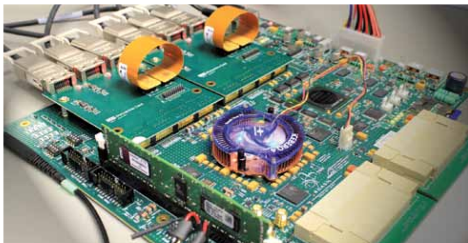
A close-up of one of the Roach II FPGA boards that will be used in the MeerKAT commissioning correlator
