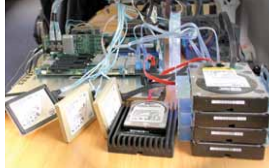
Prototype lab system, incorporating Intel solid state disk technology, used for high speed data capture and stream processing.
