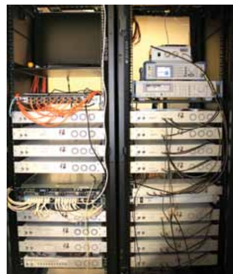
The KAT-7 laboratory correlator (a copy of the actual correlator on site to allow for complete testing of the system in a controlled environment). This correlator is based on ROACH I boards.
