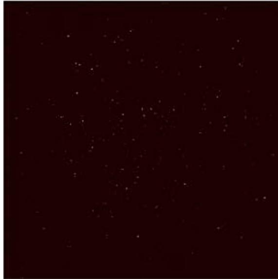
**IMAGE 1:** MeerKAT First Light image. Each white dot represents the intensity of radio waves recorded with 16 dishes of the MeerKAT telescope in the Karoo (when completed, MeerKAT will consist of 64 dishes and associated systems). More than 1300 individual objects - galaxies in the distant Universe - are seen in this image.
