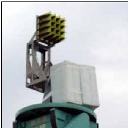
The 4x3 dual-polarized FPA mounted at the far-field antenna test range near Paardefontein, South Africa.
