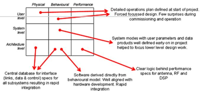
The next challenge for the systems engineering team is the Experimental Development Model (XDM) which will be a single-antenna system with full digital back-end receiver to test high-risk aspects of the KAT design. The scope of the project has been defined, based on a risk-driven strategy. Currently the XDM operations plan is being formulated which would be the major input for subsequent system design work.
