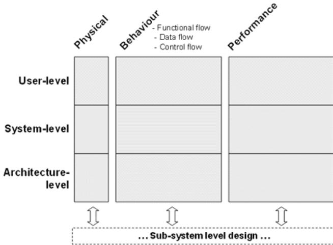
The systems engineering team must consider the physical, functional and performance aspects of the system and must trace each of these aspects from the user-level (in this case astronomer level design) through to the architecture design that will form the basis for sub-system specifications.
