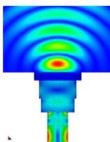
A FEKO illustration of RF currents flowing on the inner surface of the horn, and an instantaneous snapshot of the electric fields immediately outside the horn aperture.
