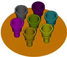
A fundamental requirement of such a horn is to exhibit a rotationally-symmetric pattern with precise control over the spatial extent, to balance the amount of wanted energy received from the dish up to its edge, compared to the unwanted noise received from the ground visible immediately outside that edge. We are quite satisfied that our design satisfies these two
