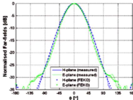
The measured far field pattern (shown here at 1 542 MHz) agrees very well with the values predicted using FEKO. These patterns will result in about a -13 dB edge taper on the 15 m prototype meerKAT dish.
