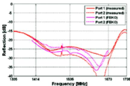
The predicted reflection coefficients agree quite well with the measured values - including the frequency of the trapped TE21L mode resonance. This resonance is caused by the asymmetry of the feed pin and was not apparent in initial coarser frequency sweeps. With the insight derived from this prototype and the agreement with numerical analyses, the next step is to remove the resonance.
