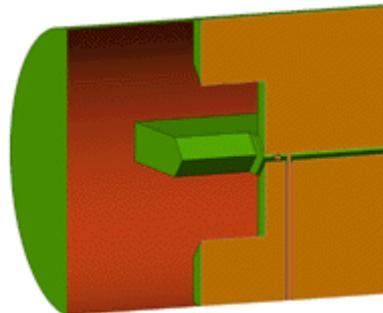
A cut through the back section of the OMT. The ridges are excited by passing a coaxial cable through the ridge and connecting the centre conductor to the opposite ridge. This high-precision pin was made by Thys Willemse, a watchmaker from On Time Watch Services in Cape Town.
