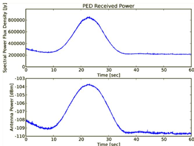
Calibrated drift scan results through the sun. Top: Measured spectral flux density versus time. Bottom: Measured power in dBm at antenna terminal. The data was calibrated by relating the received power to the LNA gain, the receiver gain, the signal bandwidth and the effective antenna area.
