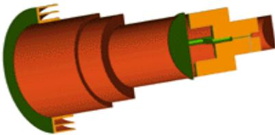
A cut through the full assembly, showing the horn, radome and quad-ridged OMT. While the model looks quite simple, it is electromagnetically quite complex. It required numerous runs of our in-house CEM software package FEKO on a SGI Altix 450 to develop the required insight into the physics of the structure.
