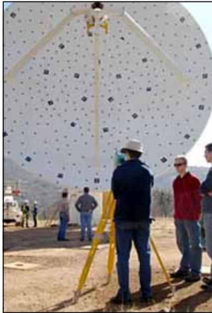
Fig 1: Theodolite and Photogrammetry measurements.
