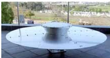
Figure 3: The floodlight antenna cavity and deflector plate (with diameter ~1500mm).
