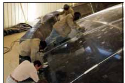
Sanding and polishing the dish mould
